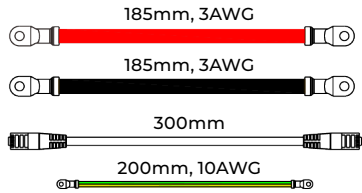
Positive parallel power cable X1 Negative parallel power cable X1 Parallel communication cable X1 Ground cable X1
